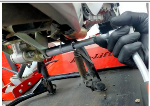
5. REMOVE THE BOLTS FROM PROLINK SYSTEM WITH TOOL 17 MM
