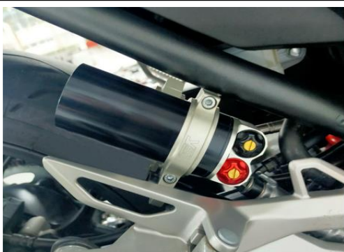
5. MOUNT THE RESERVOIR ON THE BRACKET WITH RESERVOIR CLAMP
