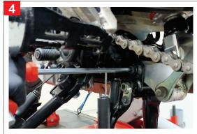
4. Assemble the Prolink and the Top and Bottom Bolts from the Shock.
