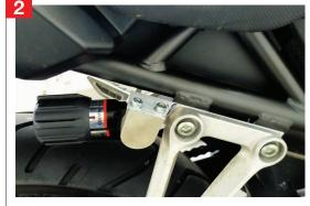
2. Mount the Hydraulic Preload Knob with the Bracket, on the Right Side of the bike.
