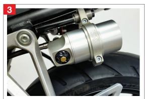
3. Mount the Reservoir with the Bracket, on the Left Side of the Bike.
