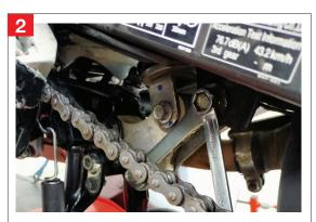
2. Take the Bolts from the Pro-Link System and the Bottom Bolt from the Original Shock out.
