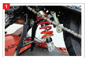
1. Assemble the YSS shock with the Reservoirs first from the Bottom to above.
