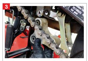
3. Take the Bolts from the Pro-Link System and the Bottom Bolt from the Original Shock out.
