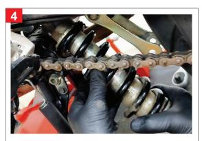
4. Take the Shock Top Bolt Out, and Remove the Pro-link System and the Original Shock.
